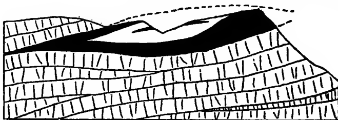
FIG. 46. Section of a composite laccolith. (After Weed and Pirsson.) The laccolith cuts heavy-bedded lava flows. Its maximum thickness is 150 feet. Black: basalt; white: granophyre.
